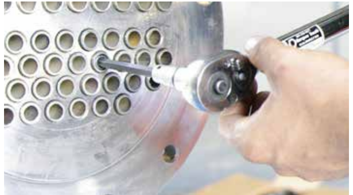
Unthread the drive screw using a hex drive.
