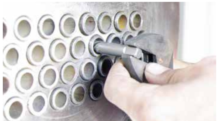
Insert an easy out tool and turn until released.
